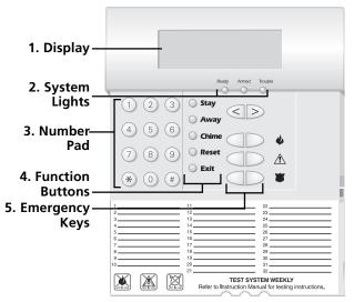
The PKP-ICON keypad shows the status of your security system using an LCD-style display, along with fixed words and numbers.
